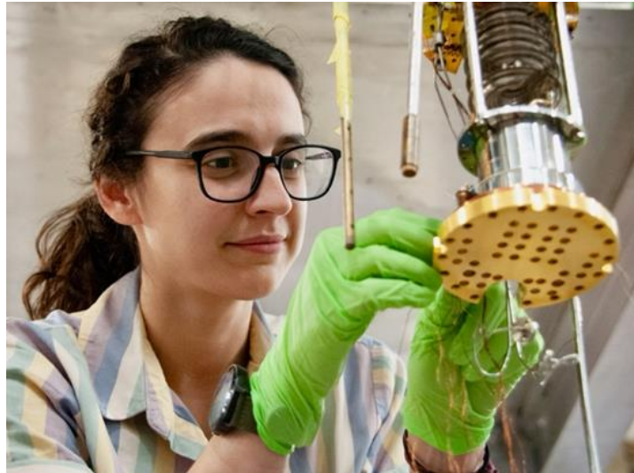
Figure 2. Dr. Mae Scott developing a low-temperature test-stand for testing of CP-TKIDs with beta sources (Image reproduced with permission from Mae Scott.)
