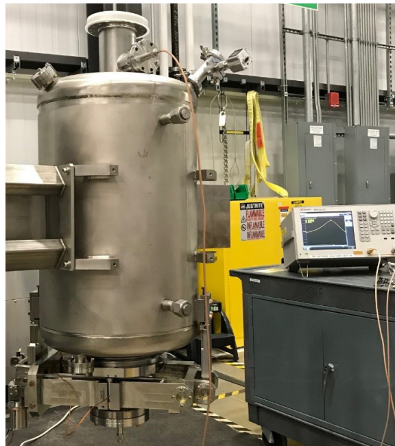
Figure 5.9: Jacketed FRIB energy upgrade cavity with the tuner installed.
