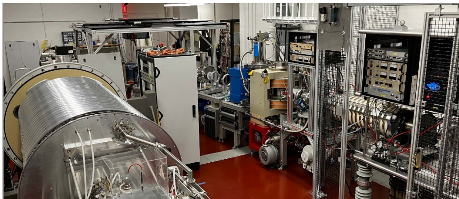
Figure 2: The new 2-MV Singletron (left) and the redesigned ECR accelerator (right) at TUNL, each machine injecting ions into a dedicated beam line. The new LENA II facility at TUNL will deliver beams of exceptionally high intensity and sharp time-structure for experiments dedicated to nuclear astrophysics.
